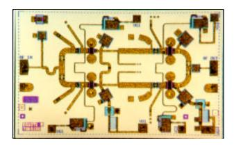
The TriQuint TGA1071-EPU is a two stage PA MMIC design using TriQuint's proven 0.25 um Power pHEMT process to support a variety of millimeter wave applications including point-to-point digital radio and point-to-multipoint systems.
