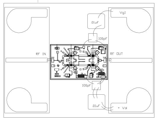
Chip Assembly and Bonding Diagram
